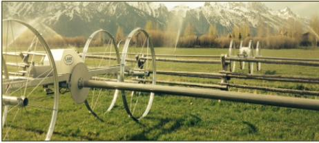
Wheel Move irrigation features an engine-driven, high pressure all-hydraulic power train.
