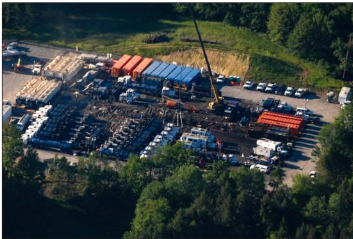
Fewer frac tanks on the pad means more space for the rest of the equipment required for a safe and successful frac job.
