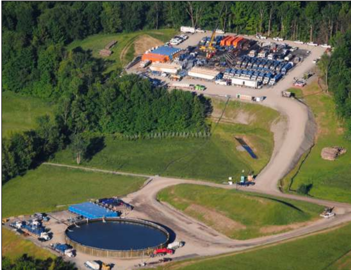
The B-40 LakeTank™ provides 40,000 barrels of water storage, economizing on hauling and labor versus standard frac tanks.
