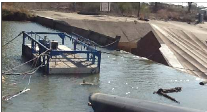
This FP1050 floating pump is capable of pumping up to 68,500 gallons per minute through a 42" discharge.
