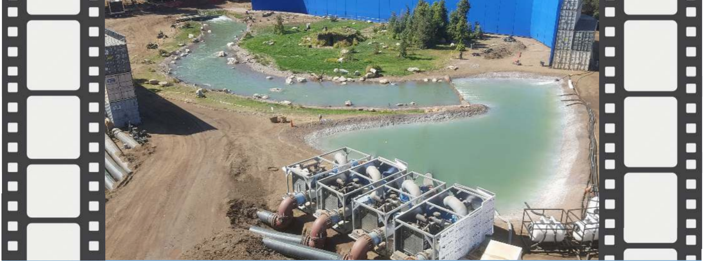
Working with the Production Co.'s Visual Effects team, Rain for Rent used four 30-inch DV600c pumps to create variable flow rates within a simulated river.
